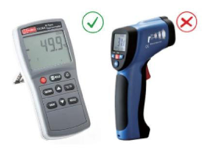
The Digital Thermometer with external probe is suitable for surface, air and immersion/penetration measurement, Laser Thermometers only measure air surfaces which can be misleading due to currents of hot air floating on the surface of the heating Element.
