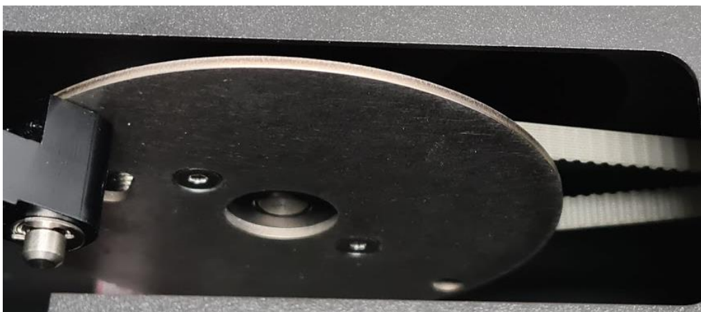
FIGURE 6-1 FLAPPER MOVEMENT MECHANISM
